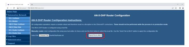
After the AN-X4 parses the router config, it will show the configuration like the screen below. There is no need to reboot the AN-X4 at this point.
