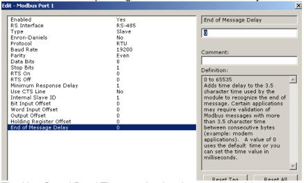
The Use Guard Band Timer setting has been removed (now assumed to be Y if you have a non-zero time out) and the Guard Band Timeout has been renamed End of Message Delay. Make the End of Message Delay equal your 5201-DFNT-MCM's Guard Band Timeout for each corresponding port. Click okay, and your conversion is complete.
