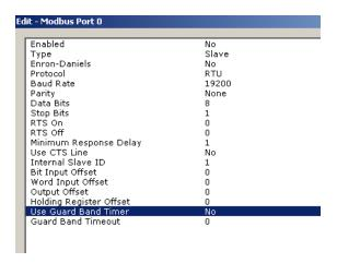
If all slave ports are set to no, or you have no slave ports, your conversion is complete. If, however, any of the Use Guard Band Timer are set to Yes, take note of the Guard Band Timeout, then corresponding Modus Port edit window in your PLX31-EIP-MBS configuration.
