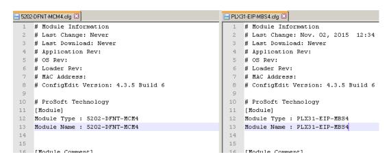
Similarly, if the Module Name field is not unique to the project, the module name field should be changed to PLX31-EIP-MBS4. This field changes the module name displayed in PCB.
