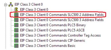
The offset into the M1 table serves as the Internal Address location within the ProSoft's memory database. Therefore, to recreate the backplane transfers shown above with Class 3 Client SLC500 2 Address Field commands, they could be configured as:
