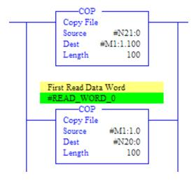
However, with the PLX gateway being a standalone unit, data transfer with the PLC program would have to be handled differently. You can recreate similar behavior with the EtherNet/IP Commands, and specifically, the Class 3 Client, SLC500 2 Address Field commands:
