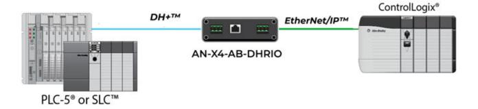
This operating mode helps the communication between an Ethernet-based processor with legacy processors on a DH+ network.
