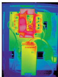
A-B 1606-XLS - 10A, 24V DC - 93% Efficiency
