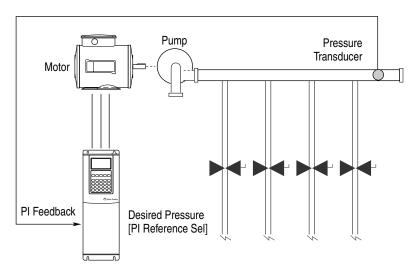
However, when additional valves in the system are opened and the pressure in the system drops, the PI error will alter its output frequency to bring the process back into control.
