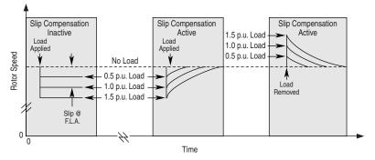
Without slip compensation active, as the load increases from no load to 150% of the motor rating, the rotor speed decreases approximately proportional to the load.
