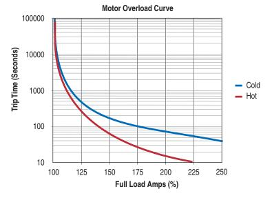
Motor nameplate FLA programming is used to set the overload feature. This parameter, which is set in the start up procedure, is adjustable from 0 - 200% of drive rating and should be set for the actual motor FLA rating.
