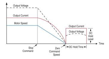
Motor speed during and after the application of DC depends upon the combination of the these two parameter settings, and the mechanical system. The drive output voltage will be zero when the hold time is finished.
