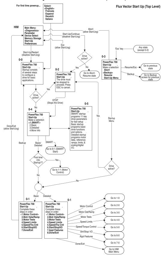
Figure 48 PowerFlex 700 Vector Control Option Startup
