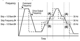
Some machinery may have a resonant operating frequency that must be avoided to minimize the risk of equipment damage. To assure that the motor cannot continuously operate at one or more of the points, skip frequencies are used. Parameters 084-086, ([Skip Frequency 1-3]) are available to set the frequencies to be avoided.
