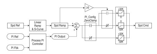
• Feedback Square Root - This feature uses the square root of the feedback signal as the PI feedback. This is useful in processes that control pressure, since centrifugal fans and pumps vary pressure with the square of speed.
