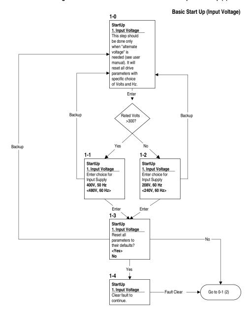
Figure 41 PowerFlex 70 & 700 Standard Control Option Startup (1)
