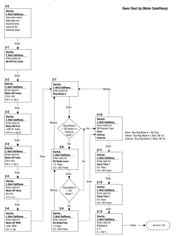
Figure 42 PowerFlex 70 & 700 Standard Control Option Startup (2)
