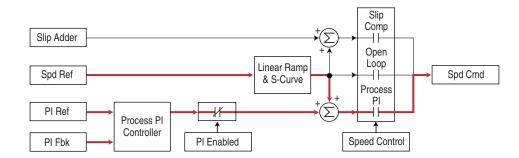
When the PI is enabled, the output of the PI Controller is added to the ramped speed reference.
