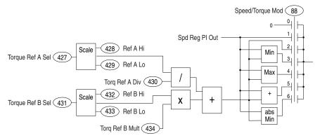
As shown, [Speed/Torque Mod] (parameter 88) is used to select the mode of operation. Zero torque current is allowed when set to "0."
