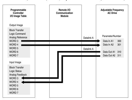
In the PLC data Table, the user enters Word 3 as a value of 100 (10.0 Secs) and word 4 as a value of 133 (13.3 seconds). On each I/O scan, the parameters in the PowerFlex drive are updated with the value from the data table: Accel Time P140 = 10.0 seconds (value from output image table Word 3) Decel Time P142 = 13.3 seconds (value from output image table Word 4).
