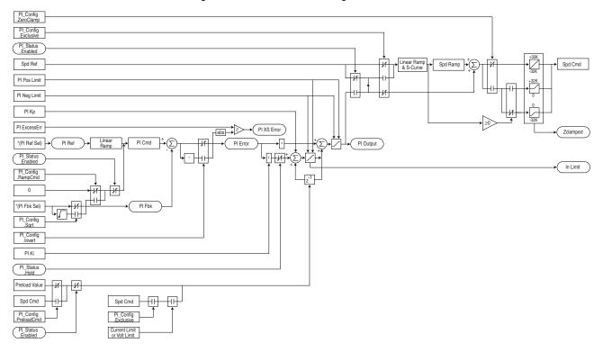
Figure 29 Process PI Block Diagram
