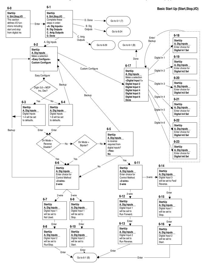
Figure 46 PowerFlex 70 & 700 Standard Control Option Startup (6)
