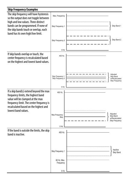
Acceleration and deceleration are not affected by the skip frequencies. Normal accel/decel will proceed through the band once the commanded frequency is greater than the skip frequency. See (A) & (B) in Figure 31. This function affects only continuous operation within the band.
