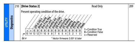
The auto-reset/run feature provides 2 status bits in [Drive Status 2] – an active status, and a countdown status.
