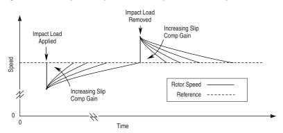
Figure 34 Rotor Speed Response Due to Impact Load and Slip Com Gain
