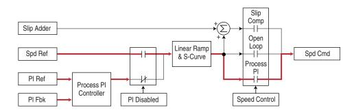
When the PI is enabled, the speed reference is disconnected and PI Output has exclusive control of the commanded speed, passing through the linear ramp and s-curve.
