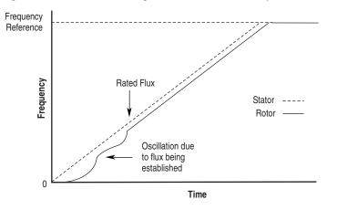
The second method is Flux Up Mode. In this mode, DC current is applied to the motor at a level equal to the lesser of the current limit setting, drive rated current, and drive DC current rating. The flux up time period is based on the level of flux up current and the rotor time constant of the motor.
