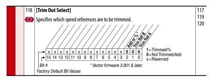
For example, % selected, Max Frequency = 130, Speed Reference = 22 Hz, Trim Reference = 20%. 4.4 Hz will be added to the Speed Reference.
