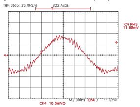
Figure 14 Current at 2 kHz PWM Frequency
