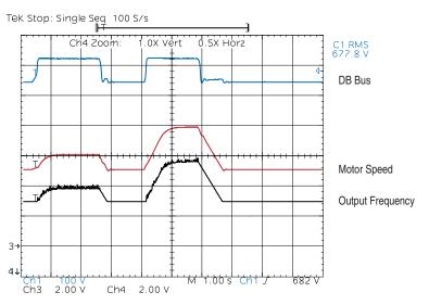
The bus voltage regulation set point (Vreg) in the drive is fixed for each voltage class of drive. The bus voltage regulation set points are identical to the internal dynamic brake regulation set points VDB's.
