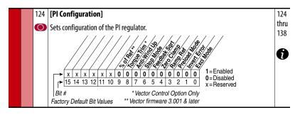
When using Process PID control the output can be selected as percent of the Speed Reference. This works in Speed trim mode only, not in Torque Trim or Exclusive Mode.
