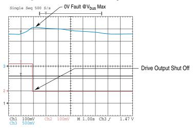
With bus regulation enabled, the drive can respond to the increasing voltage by advancing the output frequency until the regeneration is counteracted. This keeps the bus voltage at a regulated level below the trip point.
