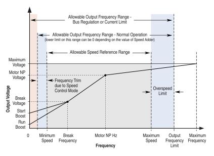
Figure 28 Typical V/Hz Curve for Full Custom (with Speed/Frequency Limits
