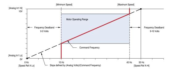
The deadband, as it relates to the analog input, can be calculated as follows:
