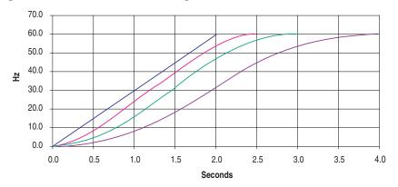
The acceleration and deceleration times are independent but the same S-curve percentage is applied to both of them. With S-curve set to 50%, acceleration time is extended by 0.5 seconds (1.0 \* 50%), and deceleration time is extended by 1.0 seconds (2.0 \* 50%).
