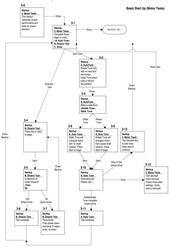
Figure 43 PowerFlex 70 & 700 Standard Control Option Startup (3)
