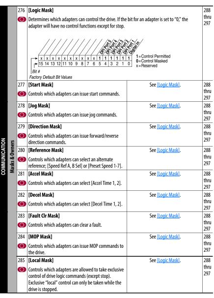
**Example:** A customer's process is normally controlled by a remote PLC, but the drive is mounted on the machine. The customer does not want anyone to walk up to the drive and reverse the motor because it would damage the process. The local HIM (drive mounted Adapter 1) is configured with an operator's panel that includes a "REV" Button. To assure that only the PLC (connected to Adapter 2) has direction control, the [Direction Mask] can be set as follows:
