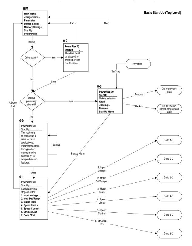
Figure 40 PowerFlex 70 & 700 Standard Control Option Startup
