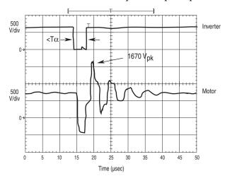
The above figure shows the inverter line-to-line output voltage (top trace) and the motor line-to-line voltage (bottom trace) for a 10 HP, 460V AC inverter, and an unloaded 10 HP AC induction motor at 60 Hz operation. 500 ft. of #12 AWG cable connects the drive to the motor.
