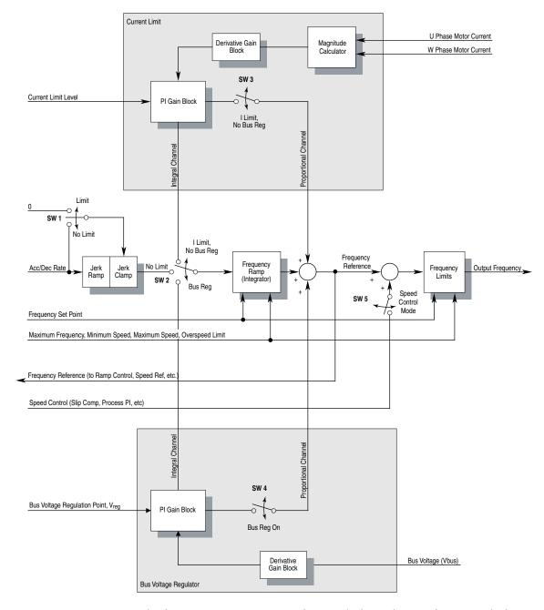
Figure 13 Bus Voltage Regulator, Current Limit and Frequency Ramp.
