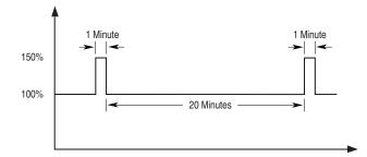
The ratio of 1:20 is the same for all durations of 150%. When operating continuous at 100%, if the load increases to 150% for 1 second the load must then return to 100% for 20 seconds before another step to 150%
