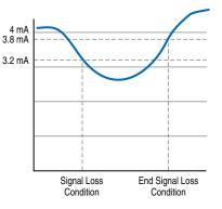
If the input is in unipolar voltage mode, 2V is the normal minimum usable input value. Any value below 1.6 volts will be interpreted by the drive as a signal loss, and a value of 1.9 volts will be required on the input in order for the signal loss condition to end.
