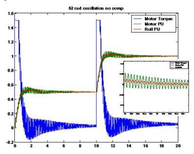
The insert shows the resonant frequency in detail.
