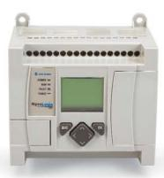
The MicroLogix 1100 combines all the features you demand in a compact controller, with EtherNet/IP messaging, online editing, a built-in LCD screen on every controller and a versatile combination of I/O.
