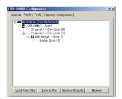
Go to the routing table configuration tab. Right-click on the DHRIO channel being used and select Add Module. Select the DH+ Bridge. Enter the DH+ node number of the KA5 (37 in this example), and the Link ID of the DH485 (13 in this example). Click Apply.
