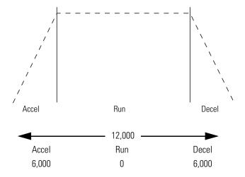
In this example, the maximum value that could be used for accelerate/decelerate is 6000, because if both accelerate and decelerate are 6000, the total number of pulses = 12,000. The run component would be zero. This profile would consist of an acceleration phase from 0 to 6000. At 6000, the output frequency (OF variable) is generated and immediately enters the deceleration phase, 6000 to 12,000. At 12,000, the PTO operation would stop (output frequency = 0).
