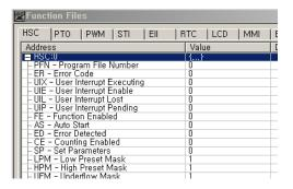
Enter the following parameters for the "Minimum Configuration" required for the HSC to count pulses.
