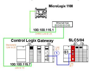
Belden 9463 "Blue Hose" cable is used to connect the DH+ devices on the network. Ethernet cable and an Ethernet hub are used to connect the ENET module and the MicroLogix 1100 CH1 Ethernet ports together.
