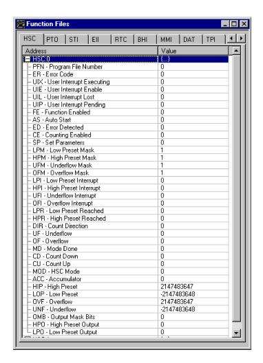
The HSC function, along with the PTO and PWM instructions, are different than most other controller instructions. Their operation is performed by custom circuitry that runs in parallel with the main system processor. This is necessary because of the high performance requirements of these functions.
