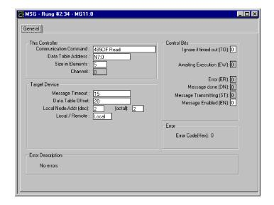
In this example, the controller reads five elements (words) from the target device's (Local Node 2) CIF file, starting at word 20 (or byte 20 for non-SLC 500 devices). The five elements are placed in the controller's integer file starting at word N7:0. If 15 seconds elapse before the message completes, error bit MG11:0/ER is set, indicating that the message timed out.
