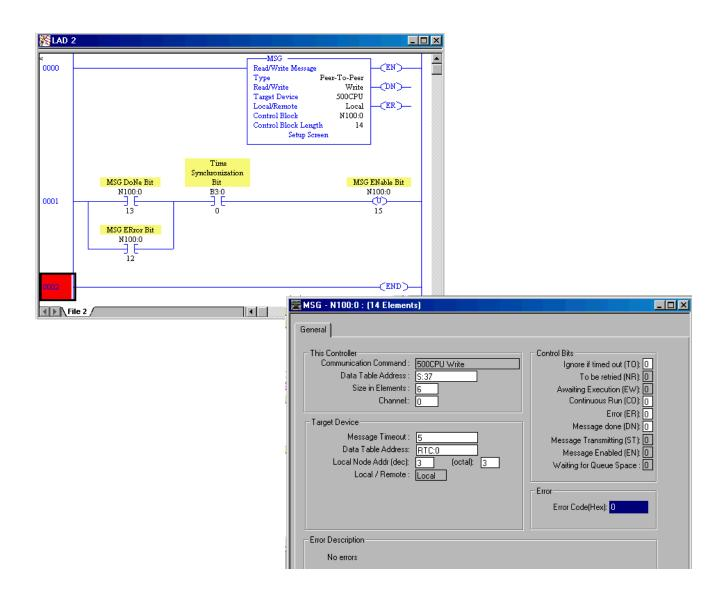
The example above messages the SLC 500 Date and Time data (S:37 - S:42) to the MicroLogix 1100 RTC, each time the SLC processor is powered up and placed into the RUN mode or each time the Time Synchronization Bit (B3:0/0) is enabled.
