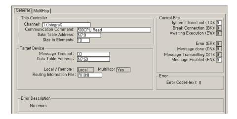
In this example, the controller reads 10 elements from the target's N7 file, starting at word N7:50 using 500CPU Read command. The 10 words are placed in the controller's integer file starting at word N7:0. If 33 seconds elapse before the message completes, error bit MG11:0/ER is set, indicating that the message timed out.
