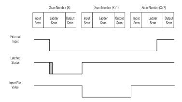
**TIP** The "gray" area of the Latched Status waveform is the input filter delay.
