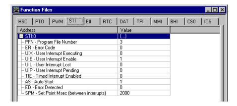
IMPORTANT: Ladder Logic Subroutine file #3 must be created in order for this example to work. If the subroutine is not created the CPU will fault due to a STI Error Code 1 - Invalid File Number for PFN has been entered.
