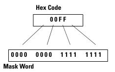
Bits of the mask word that are set (1) will pass data from a source to a destination. Reset bits (0) will not. In the example below, data in bits 0-7 of the source word is passed to the destination word. Data in bits 8-15 of the source word is not passed to the destination word.
