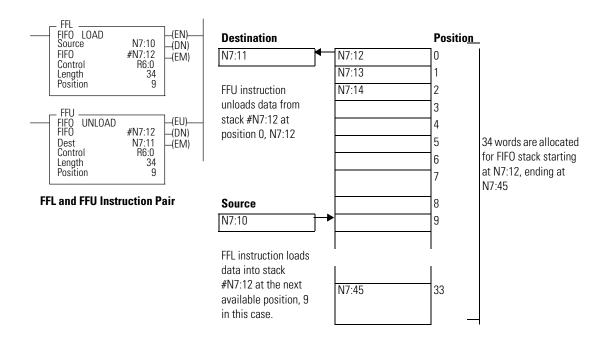
Loading and Unloading of Stack #N7:12
