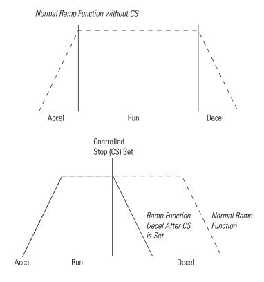
If the CS bit is set during the accel phase, the accel phase completes and the PTO immediately enters the decel phase.
