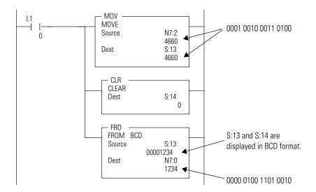
When the input condition I:0/1 is set (1), a BCD value (transferred from a 4-digit thumbwheel switch for example) is moved from word N7:2 into the math register. Status word S:14 is then cleared to make certain that unwanted data is not present when the FRD instruction is executed.
