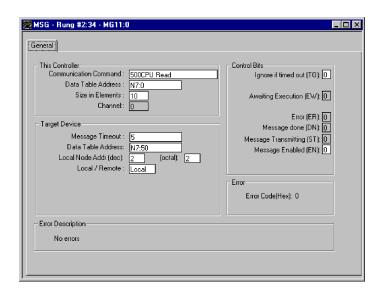
In this example, the controller reads 10 elements from the target's (Local Node 2) N7 file, starting at word N7:50. The 10 words are placed in the controller's integer file starting at word N7:0. If five seconds elapse before the message completes, error bit MG11:0/ER is set, indicating that the message timed out.
