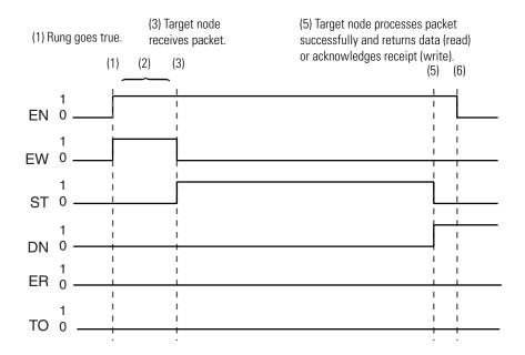
1. If there is room in any of the four active message buffers when the MSG rung becomes true and the MSG is scanned, the EN and EW bits for this message are set. If this is a MSG write instruction, the source data is transferred to the message buffer at this time.
