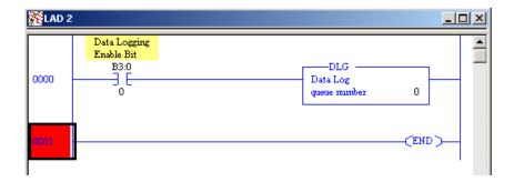
FYI - The DLG instruction ONLY captures data on a false-to-true rung transition.
