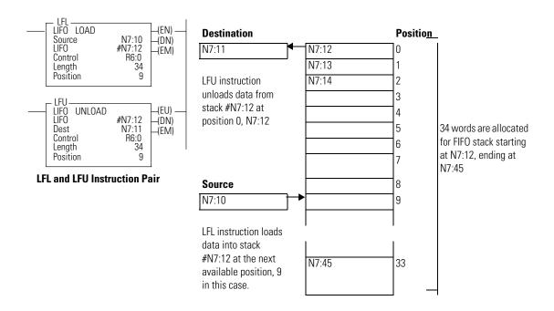
Loading and Unloading of Stack #N7:12
