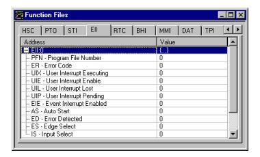
Each EII can be configured to monitor any one of the first eight inputs (I1:0.0/0 to I1:0.0/7). Each EII can be configured to detect rising edge or falling edge input signals. When the configured input signal is detected at the input terminal, the controller immediately scans the configured subroutine.
