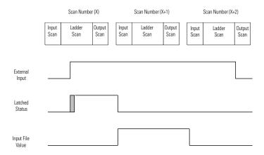
**TIP** The "gray" area of the Latched Status waveform is the input filter delay.
