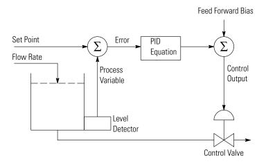
The PID equation controls the process by sending an output signal to the control valve. The greater the error between the setpoint and process variable input, the greater the output signal. Alternately, the smaller the
