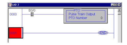
By toggling Bit B3/0 the PTO can be activated. Once running the PTO will generate the number of pulses entered into the PTO:0.TOP word and then stop. To restart, toggle B3/0.
