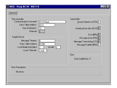
In this example, the controller reads 10 elements from the target device's (Local Node 2) N7 file, starting at word N7:50. The 10 words are placed in the controller's integer file starting at word N7:0. If five seconds elapse before the message completes, error bit MG11:0/ER is set, indicating that the message timed out.
