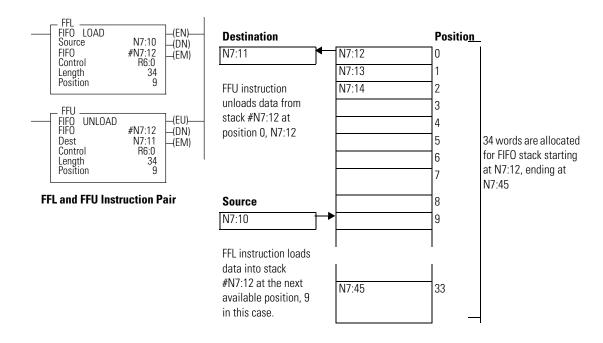
Loading and Unloading of Stack #N7:12
