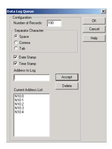
**IMPORTANT NOTE** - Integer file N10 must be created with a length of 5 or the software will not compile the ladder program. Also an embedded RTC must be enabled and configured if the Date and Time stamp are to be used. If an RTC module is disabled the data for these fields will contain zeros.
