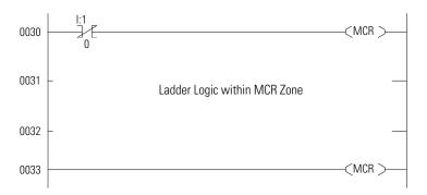
While the rung state of the first MCR instruction is true, execution proceeds as if the zone were not present. When the rung state of the first MCR instruction is false, the ladder logic within the MCR zone is executed as if the rung is false. All non-retentive outputs within the MCR zone are reset.
