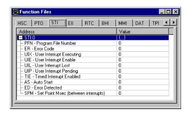
The Selectable Timed Interrupt (STI) provides a mechanism to solve time critical control requirements. The STI is a trigger mechanism that allows you to scan or solve control program logic that is time sensitive.
