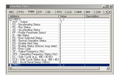
Enter the following parameters as the "Minimum Configuration" required for the PWM to generate a waveform at the specified frequency.
