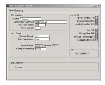
A MSG route must be configured in the MultiHop tab of the MSG Setup Screen.
