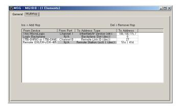
Enter in the IP address of the 1756 ENET module, select ControlLogix backplane, press the Insert key and enter in the backplane slot numbers of the DHRIO module (0-16) under the 'To Address' fields. Click on the ControlLogix backplane to highlight it and press the Insert key on your computer's keyboard to add another hop. Double click on the From Device under the ControlLogix backplane and select the 1756-DHRIO. Make sure that the From Port for the DHRIO module is set for Channel B.
