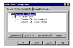
Right click on the Backplane and left click on Edit Module. Make sure that the Back plane Link ID is set to 20.
