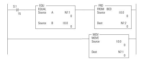
The two rungs shown cause the controller to verify that the value I:0 remains the same for two consecutive scans before it executes the FRD. This prevents the FRD from converting a non-BCD value during an input value change.
