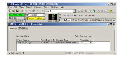
Trigger MSG instruction. It should complete done, and OPC Test Client should display the N7:0 data, as well as "Good" Sub Quality:
