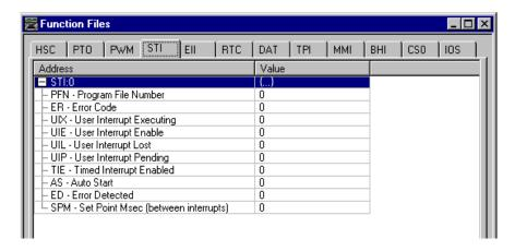
Enter the following parameters as the "Minimum Configuration" required for the STI
