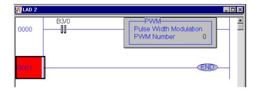
By toggling Bit B3/0 the PWM can be activated.
