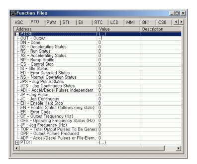
Enter the following parameters as the "Minimum Configuration" required for the PTO to generate pulses.
