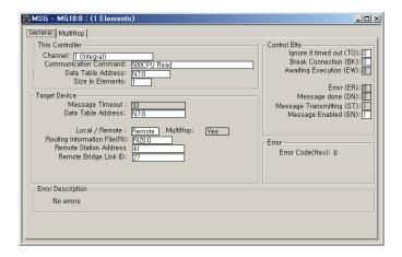
A MSG route must be configured in the MultiHop tab of the MSG Setup Screen. Click on the MultiHop tab.
