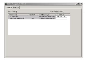
Enter in the IP address of the 1756 ENET module, select ControlLogix backplane, press the Insert key and enter in the backplane slot numbers of the DHRIO module (0-16) under the 'To Address' fields.
