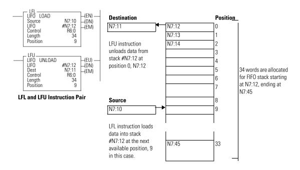
Loading and Unloading of Stack #N7:12
