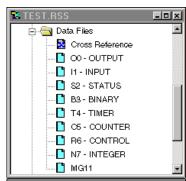
The MSG instruction built into the controller uses a MG data file to process the message instruction. The MG data file, shown at left, is accessed using the MG prefix. Each message instruction utilizes an element within a MG data file. For example, MG11:0 is the first element in message data file 11.
