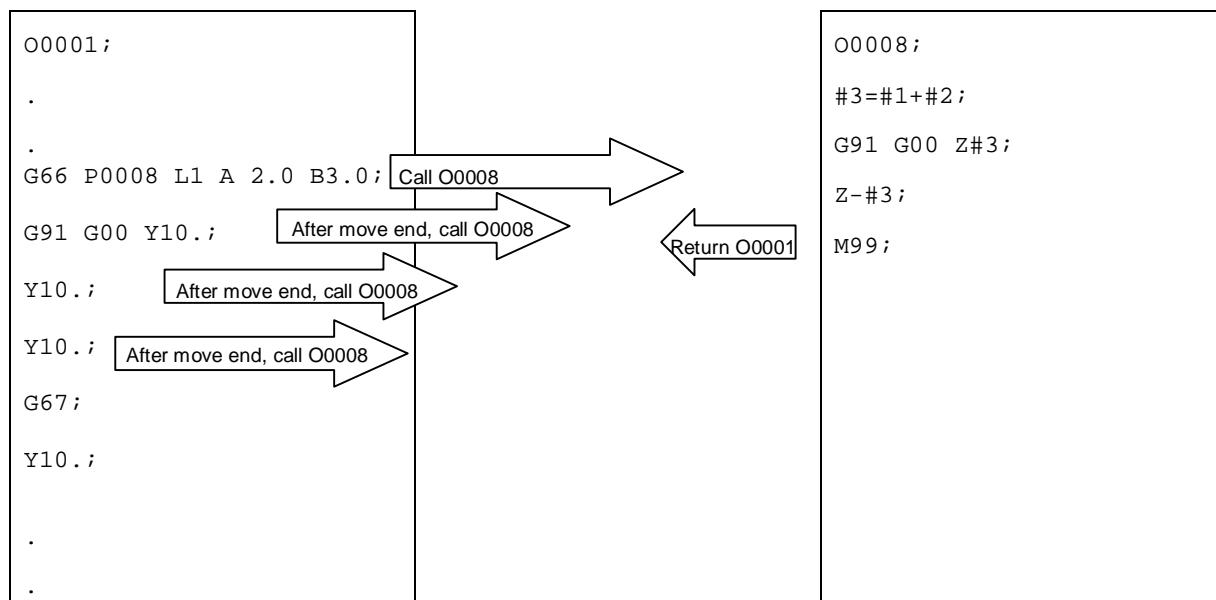
In a G66 block, G66 must be prior to all arguments. G66 can do nested calls. The combination of G65 and G66 can be up to the 4<sup>th</sup> level (excluding main program which is the 0<sup>th</sup> level), but G66's argument (corresponding to macro program's local variables) is only specified once in the block of G66, and it won't be respecified in following mode calls.
