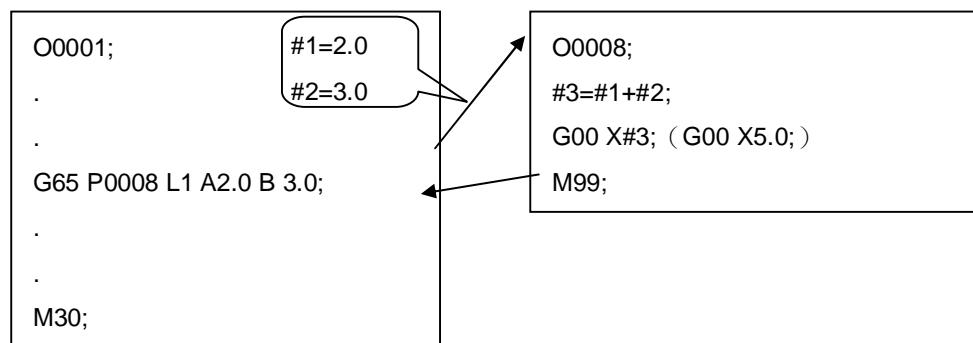
In a G65 block, G65 must be prior to all arguments. G65 can do nested calls, the combination of G65 and G66 can be up to the 4<sup>th</sup> level (excluding main program which is the 0<sup>th</sup> level), and each level has its own local variables, as shown in the following charts:
