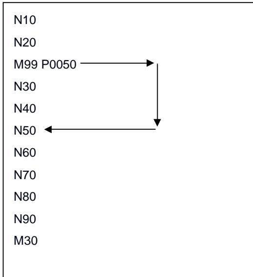
If use M99 P\_\_ in the end of subprogram, when subprogram ends and system returns to main program, system continues executing from the line specified by M99.
