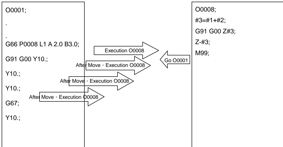
In G66 blocks, G66 must be written before all arguments. Like G65, the nest type call could be done by G66, and up to 4 levels are available for the combination of G66 and G65, (The main program is not included, and the main program is level 0), but the G66 arguments (corresponding to local variables of macro program) can only be set for once in G66 block, and then the mode calling will not be reset aincemental.
