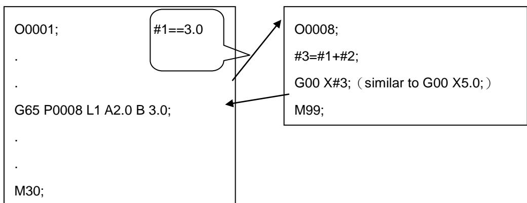
In G65 blocks, G65 must be written before all arguments. The nest type call can be done towards G65, and up to four levels are available for the combination of G65 and G66 (The main program is
