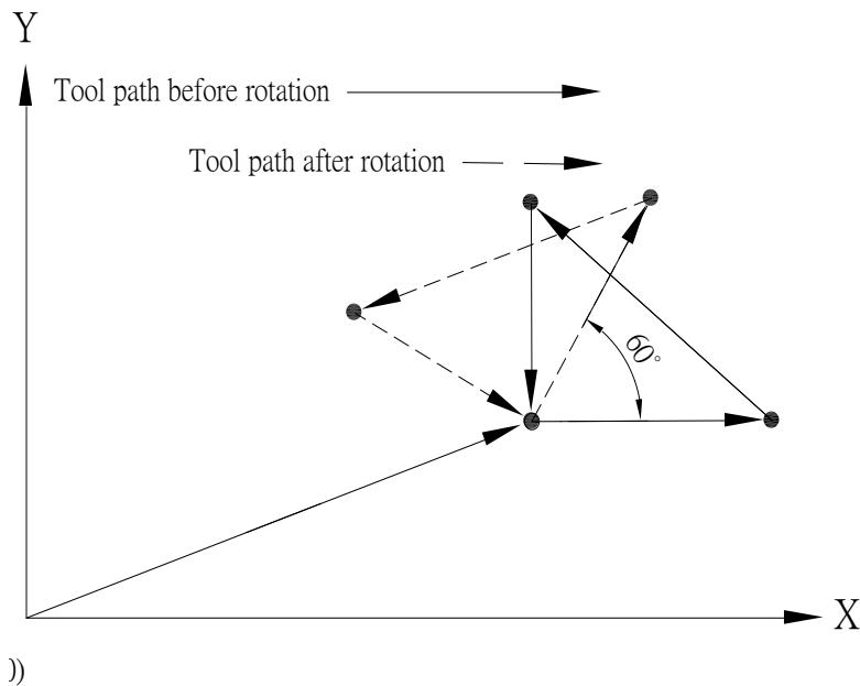
If the moving block subsequent to G68 is incremental mode (G91), the current position of G68 will be considered as the rotation center.
