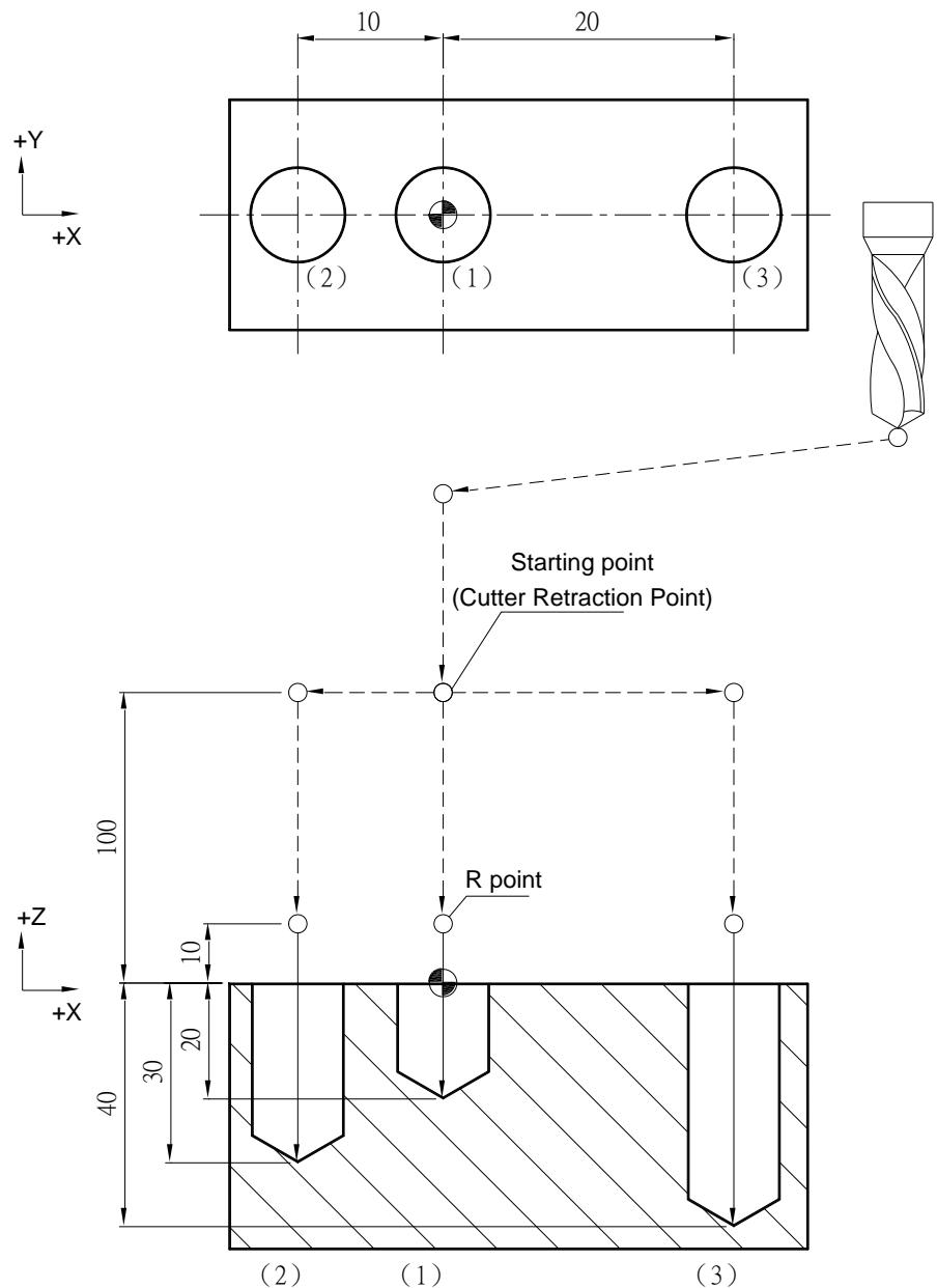
**G74 Left-Handed Screw Thread Tapping Cycle****Command Format**
