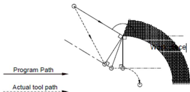
**G43, G44, G49 Tool Length Compensation****Command Format**
