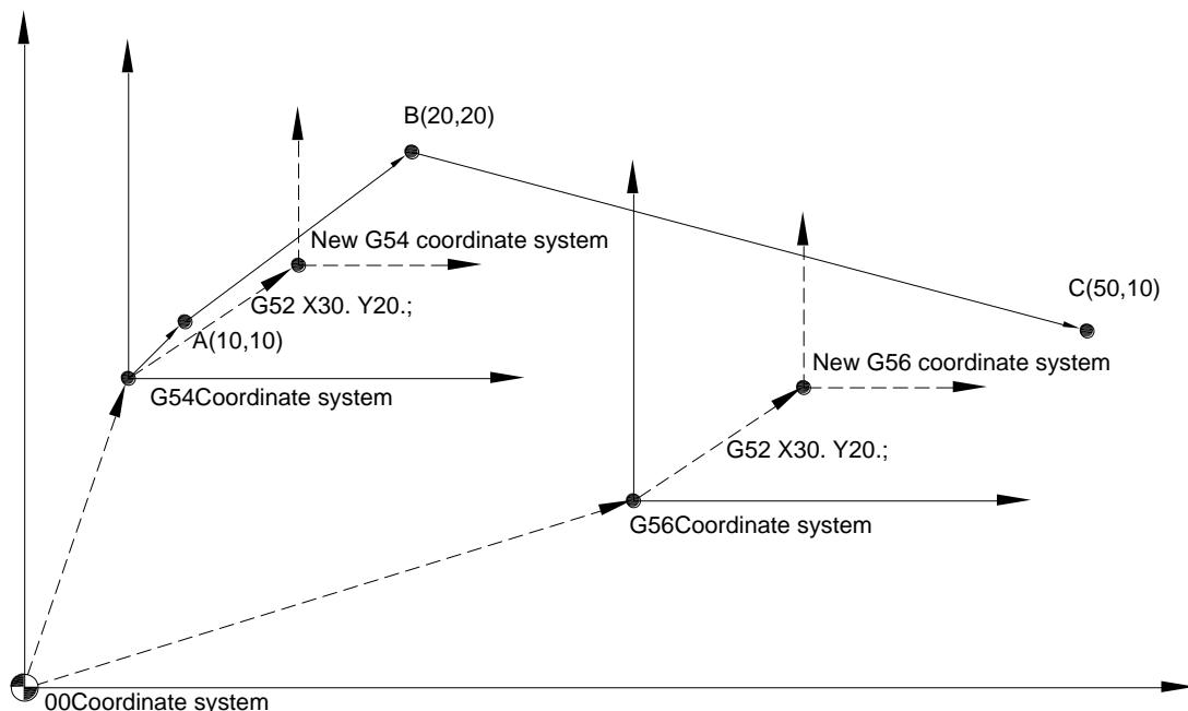
There are two methods to cancel the interval coordinate system set by G52. The first method is to run “manually return to origin” procedure (and parameter #0133 is set to 1); the second method is to run G52 command a incremental, but the argument being used must be the negative value of the argument used by G52 command at the last time.
