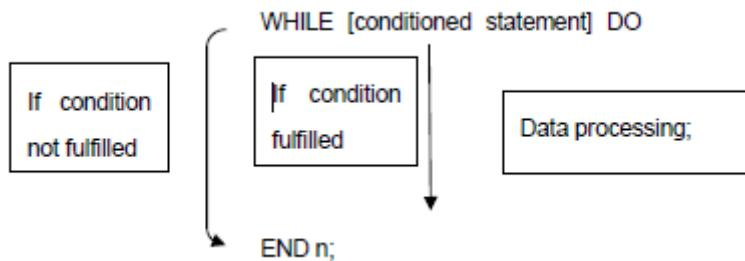
Sequential numbers after DO and END are identification symbols of execution range. Use 1, 2, 3 as the identification number. If numbers other than 1, 2, 3 are used, system alarm #3170 will be triggered in the Do statement as:  $1 \leq n \leq 3$  unsatisfied.
