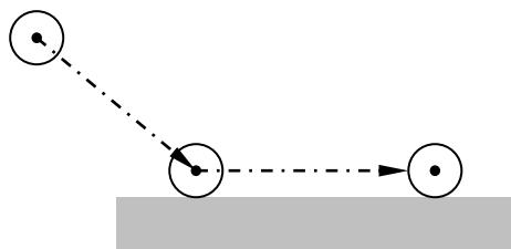
G42 : The tool has an offset of an amount of the radius to the right when facing to the direction of the tool movement.
