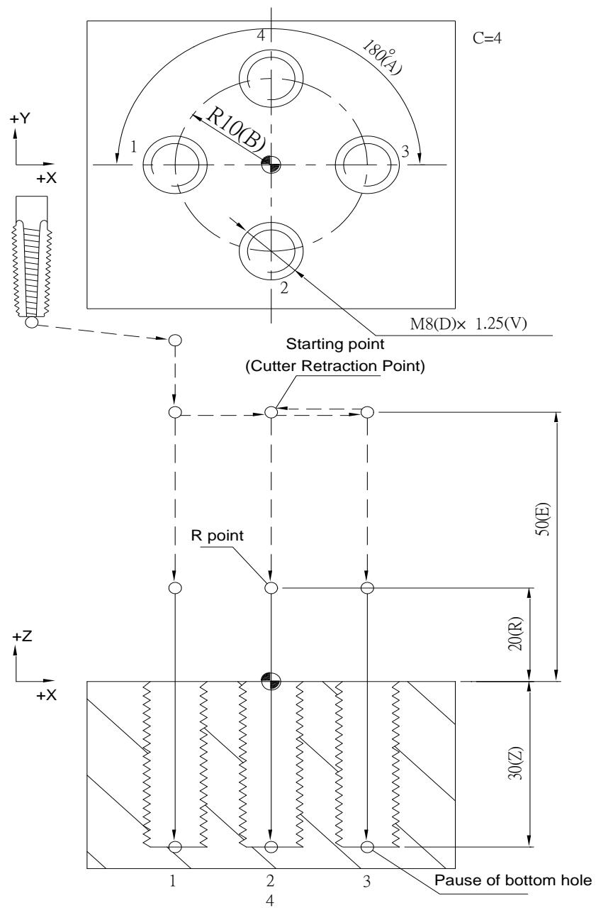
**G103 Arc Mode of Multi-hole Manufacturing Cycle****Command Format**
