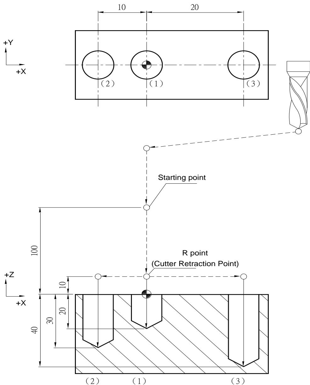
**G84 Right-Handed Screw Thread Tapping Cycle****Command Format**
