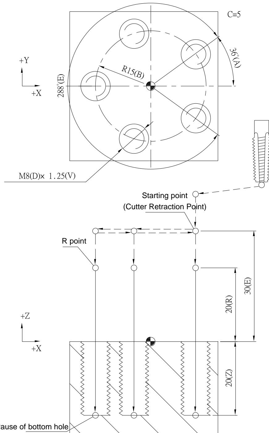
**G104 Grid Mode of Multi-hole Manufacturing Cycle****Command Format**
