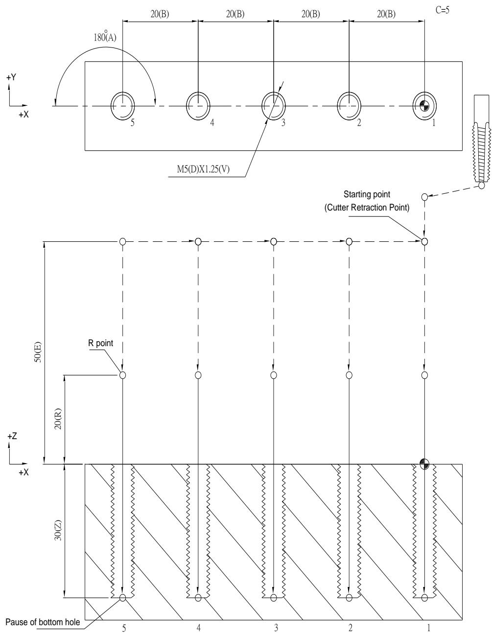
**G102 Circular Mode of Multi-hole Manufacturing Cycle****Command Format**
