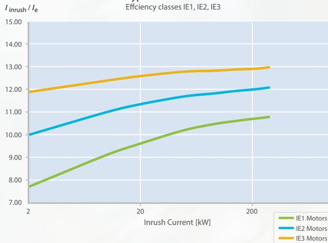
The specific starting current characteristics of the higher efficiency motors are requiring a special attention. A proper selection of the motor starting and switching components will make sure that the application starts without disturbances nor component damages. In particular, the following risks exist and must be avoided:
