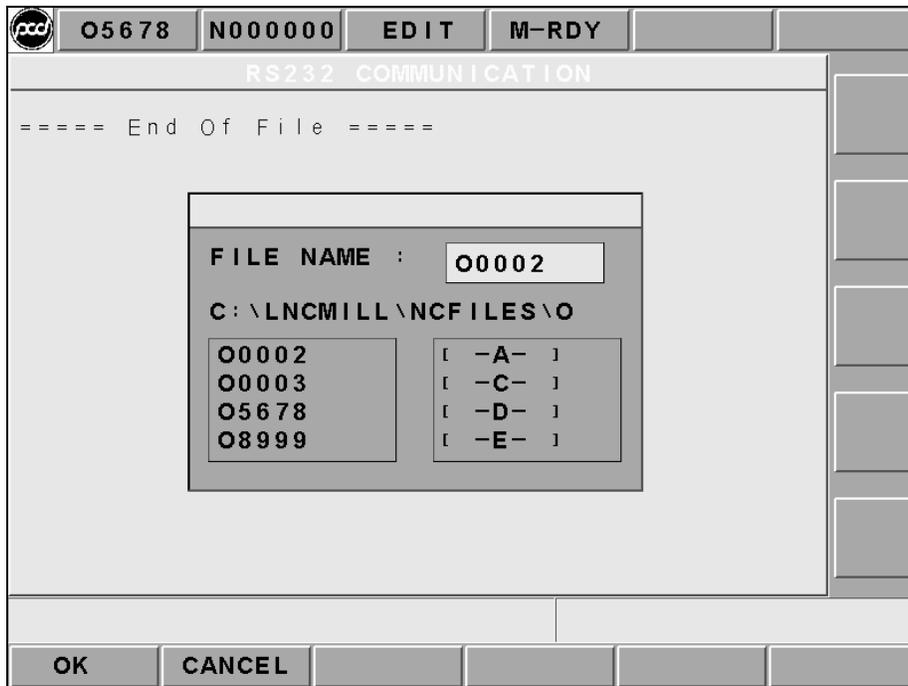
Figure 2.5-26 Selecting File Transmitting Function Screen
