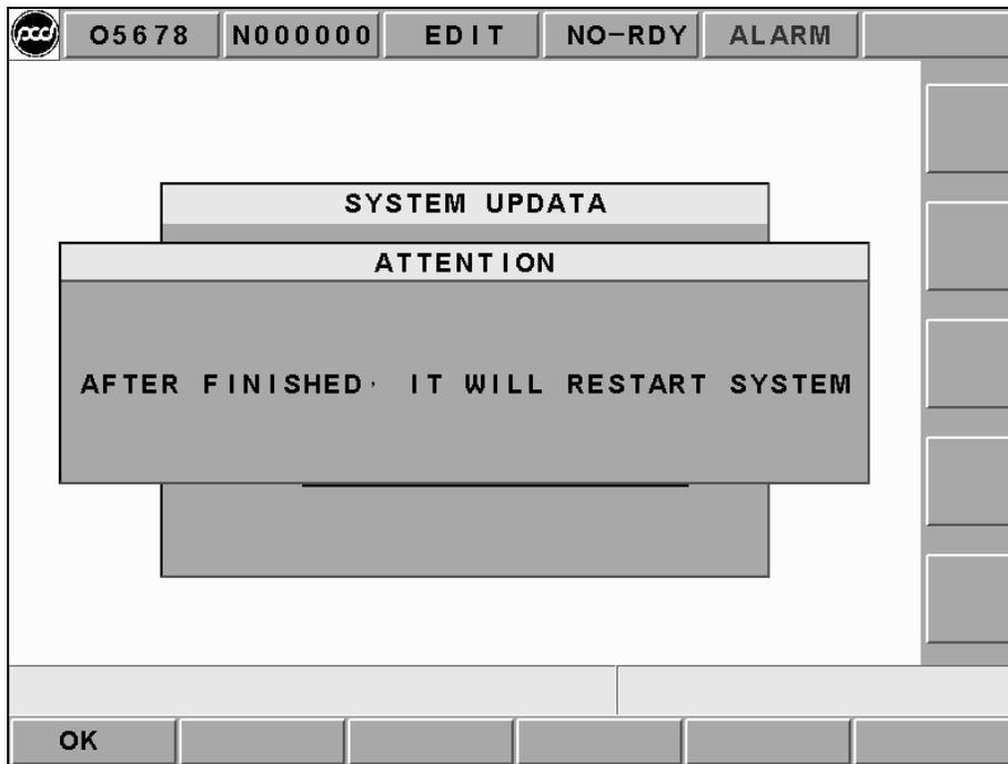
Figure 2.9-6 Reminding Users to Reboot after Key-In Parameter
